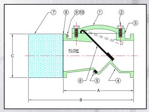
the valve from the line. The Elastic Swing Foot Valve is designed for continuous flow applications and is not recommended for reciprocating pumps. The Elastic Swing Foot Valve can be installed in a vertical or horizontal pipeline.
