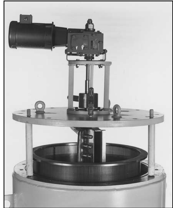
Figure 2 - The innovative internals of the Hyper-Jet ™ showing ease of maintenance.
